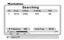
Shows serial number of TP, Frequency, Symbol Rate (S/R), Polarity and FEC found.
